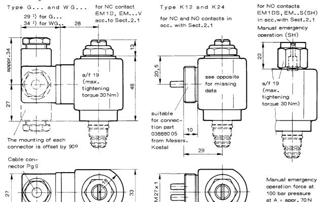
$^{1}$ ) These dimensions are possible up to max. 40 mm depending on the make (here Messrs. Klar und Beilschmidt, Landshut) in accordance with DIN 43 650
